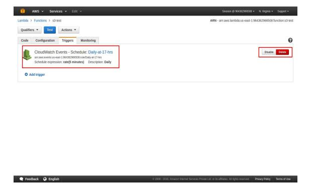
**Note**: We can run the Lambda function by adding triggers, we need to disable, when we have multiple versions, because triggers run automatically in backend. We can monitor the lambda function through cloud-watch.
